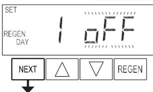
**Step 3I** - Scroll through days 1 to 7 using NEXT. Use ▲ or ▼ to turn regen ON or OFF for each individual day. After completing the 7th day, press NEXT to go to Step 4I. Press REGEN to go to previous display.
