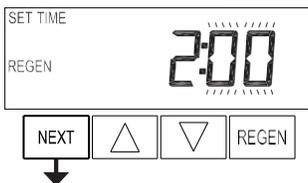
**Step 5I** - Next Regeneration Time (minutes): Set the minutes of day for regeneration using ▲ or ▼. Press NEXT to exit Installer Display Settings. Press REGEN to return to previous step.
