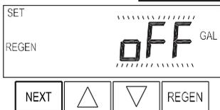
**Step 5F** - Set Regeneration trigger using ▲ or ▼. If value is set to:
