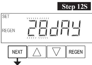
**Step 12S** – Set Regeneration Trigger using ▲ or ▼. If Step 11S is set to OFF, Regeneration Trigger can be set to 28 day or 7 day. Press NEXT to go to Step 13S. Press REGEN to return to previous step.
