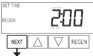
**Step 4I** - Next Regeneration Time (hour): Set the hour of day for regeneration using ▲ or ▼. The default time is 2:00. Press NEXT to go to step 5I. Press REGEN to return to previous step.
