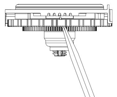
The drive cap assembly contains the drive cap, the main drive gear, drive cap spline, piston rod and various other parts that should not be dissembled in the field. The only replaceable part on the drive cap assembly is the O-ring. Attached to the drive cap assembly is the main piston (downflow or upflow) and if a regenerant is used, a regenerant piston.
