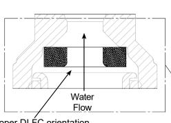
Proper DLFC orientation directs water flow towards the washer face with rounded edge.
