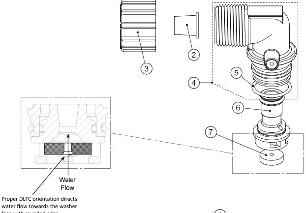
water flow towards the washer face with rounded edge.
