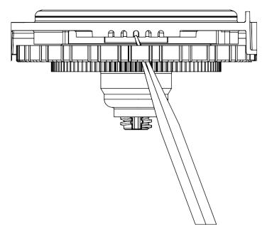
The drive cap assembly contains the drive cap, the main drive gear, drive cap spline, piston rod and various other parts that should not be dissembled in the field. The only replaceable part on the drive cap assembly is the O-ring. Attached to the drive cap assembly is the main piston (downflow or upflow) and if a regenerant is used, a regenerant piston.
