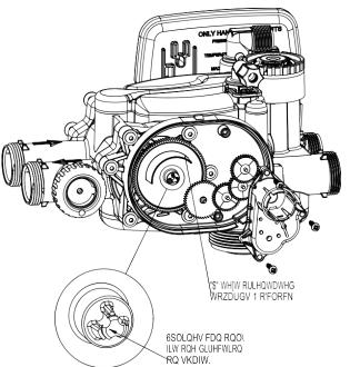
Noting the one possible orientation of the transfer drive cap, use one hand to press in and support the transfer drive cap while using the opposing hand to start two screws in, one on the top and one opposing it on the bottom. Tighten the screws in evenly so the cap seats the O-ring without getting pinched or damaged. Screws should only be hand tightened with a 5/32" or 4mm Allen Wrench, **DO NOT OVER TIGHTEN SCREWS.**
