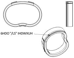
transfer discs may be removed by pulling the discs outward off of the shaft away from the valve body with your hand. With the disc out you can inspect the flat surface area to be sure it's clean and smooth free of any debris or scratches. Note that the disc is keyed to the drive shaft so that it will only assemble in one orientation. The transfer discs may be chemically cleaned with a dilute sodium bisulfate solution, vinegar or just wiped with a soft clean cloth.
