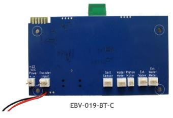
The valve board wiring connections are labeled clearly according to their function. "Salt Sensor", "Ext. Valve" and "Ext Water Meter" are for future use and for now should not be connected to.
