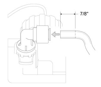
To release the brine tubing from the brine port on the valve:
